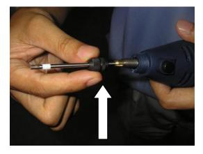
Put collar onto the shaft and screw it back to the drive itself! While doing that you
