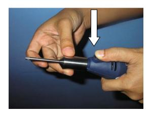
Press the black locking button and screw it fully onto the drive!
